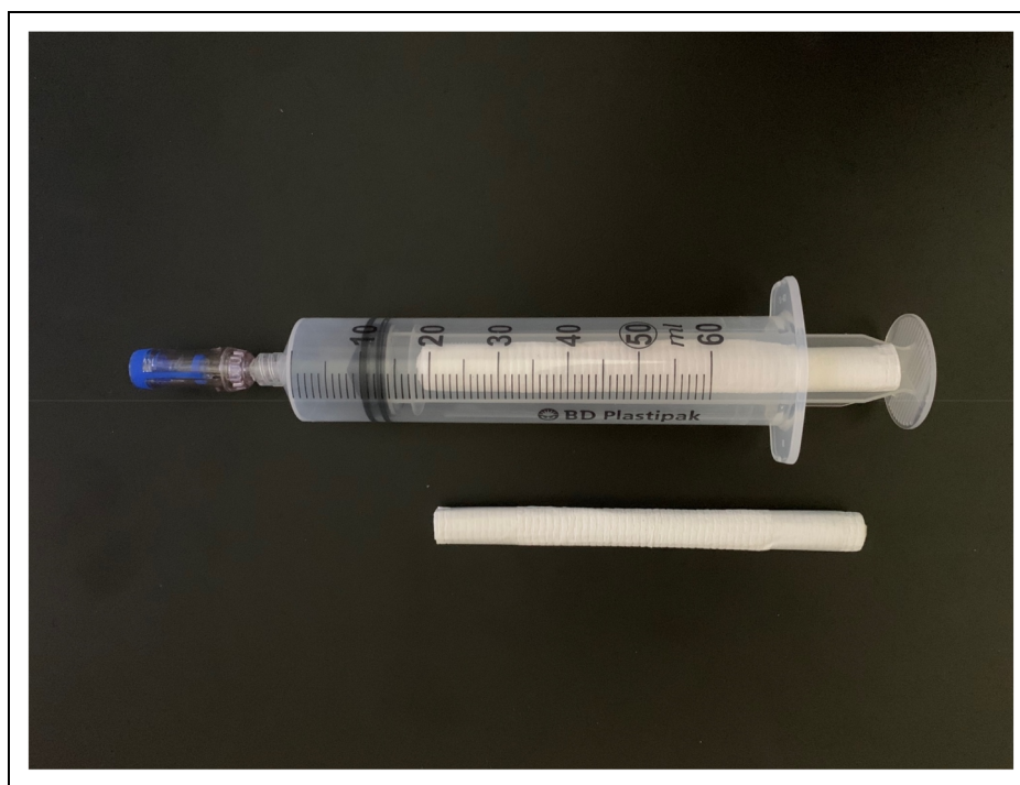
Figure 1. Cylinder-shaped wipe and syringe with cylinder-shaped wipe inside the barrel.
