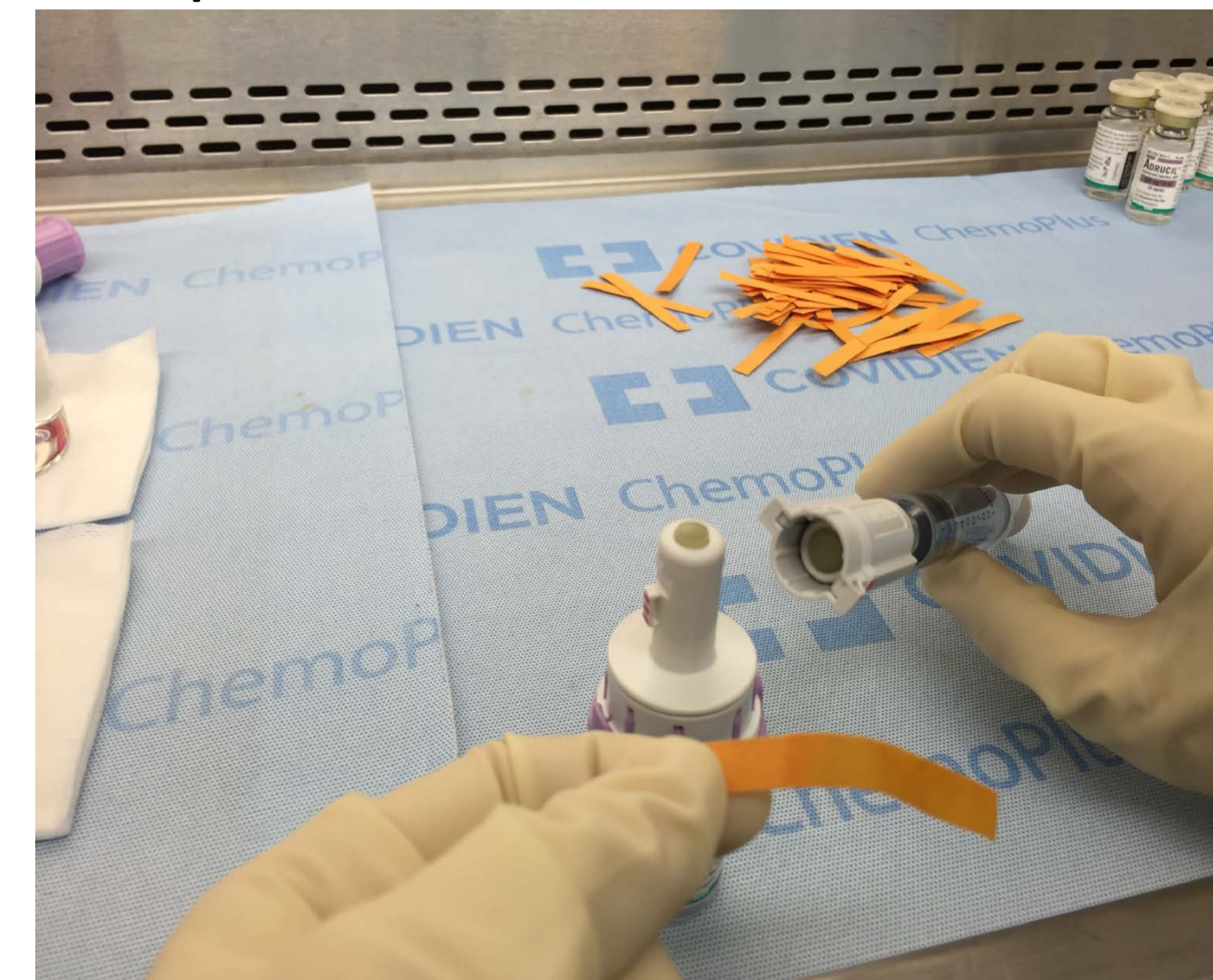
FIGURE 3. Equashield® demonstrating no leakage in the syringe and vial connector during a sample run.
