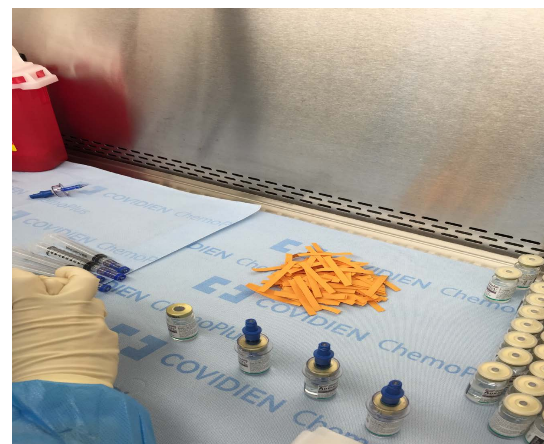
FIGURE 1. Separate syringes and vials were fitted with the CSTD being tested before manipulation of 5-FU.
