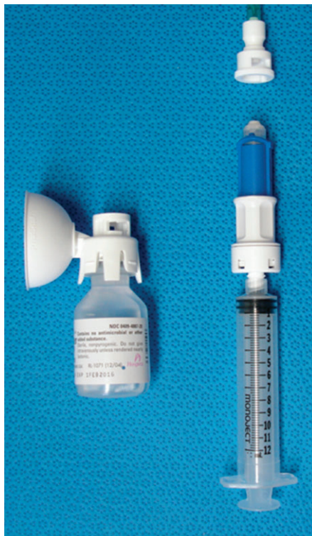
Figure 1. PhaSeal® closed system transfer device. The three main components are the protector (left), injector (bottom right) and connector (top right). The injector contains a needle enclosed within a protective sleeve sealed by a double membrane. It attaches to a syringe or IV tubing. The protector is a drug vial adaptor with a flexible expansion bulb that is permanently attached to the vial and used for closed drug reconstitution and pressure equalization. The connector attaches to an IV catheter to provide a closed connection with the injector.
